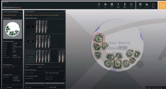
Fig. 16: The mandibular restorations in the Prettau® Anterior® zirconia block. In the nesting software, it is possible to preview the burs' milling paths.
