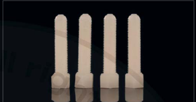
Fig. 17: The sealing screws milled out of the resin Screw Blank.
