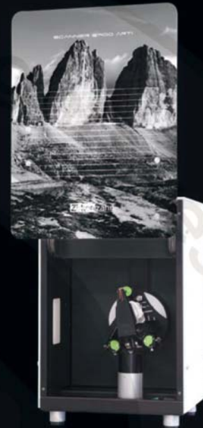
Fig. 9: The digitalisation of the maxillary and mandibular models, as well as the registration of the articulator were performed with the new S900 ARTI scanner. This new scanner is equipped with 3 cameras, for a particularly high scan data density and depth detection.
