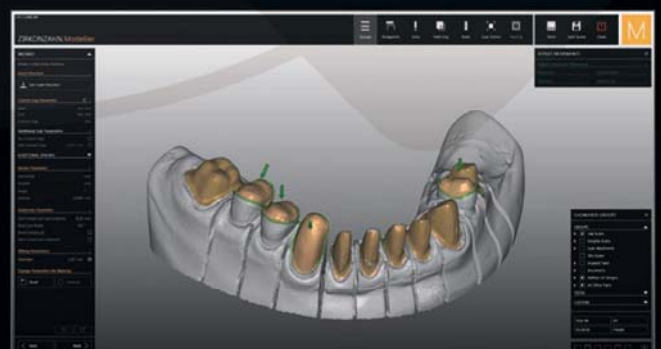
Fig. 15: The definition of the insertion axis in the mandibular restoration.
